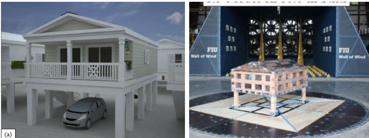
Figure 4: Rendering of the subject elevated structure (left) and 1:5 scale model on WOW turntable (right) (from Chowdhury et al. 2017)
