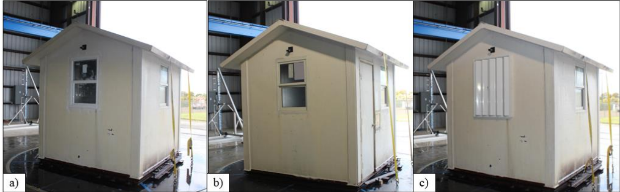
Figure 2 Window and shutter test configurations: a) Nonimpact window, b) Impact-resistant window, and c) Accordion shutter (installed over nonimpact window).
