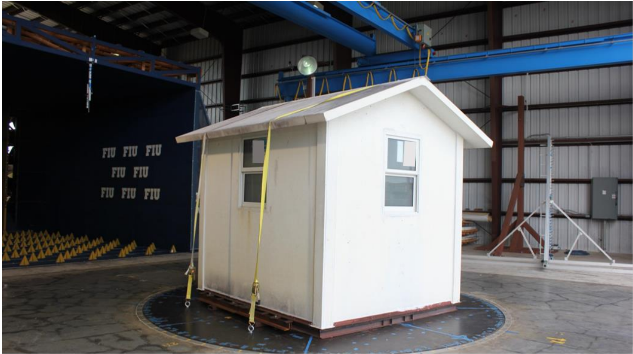
Figure 1 Large-scale SIP building model installed on WOW turntable.
