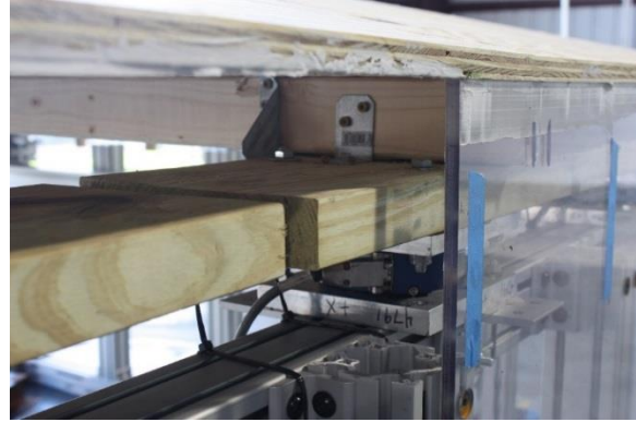
Figure 2: 1:4 scale model on WOW turntable (left). Installed load cell at r2w connection (right) (source: FIU)
