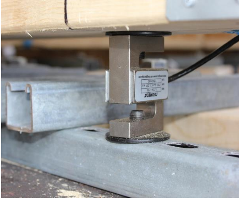
Figure 17: Load cell anchored to ground using uni-strut braces
