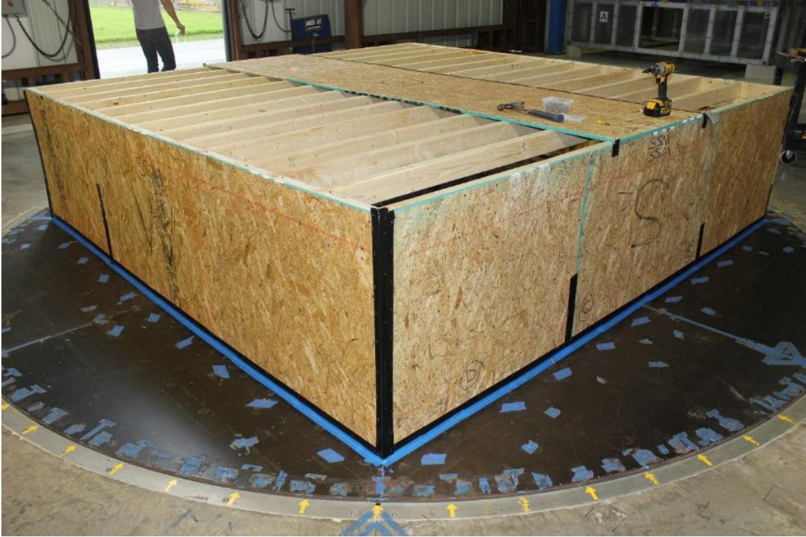
Figure 6: SSM model with wall sheathing attached, SW corner
