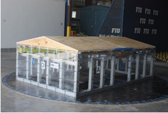
Figure 2: 1:4 scale model on WOW turntable (left). Installed load cell at r2w connection (right) (source: FIU)
